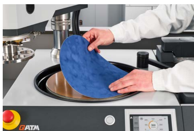
Placing e.g. self-adhesive polishing cloth on GALAXY X-Tap
