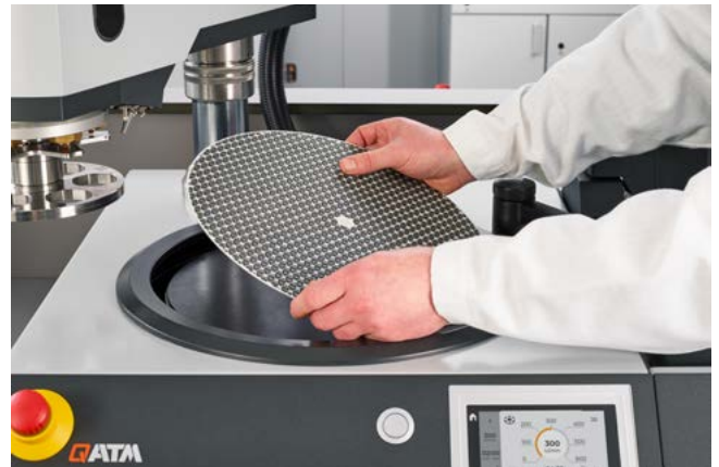
Placing e.g. a diamond grinding disc on the magnetic foil
